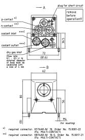
\*\*) required connector: KBT6AR-N/ 10-S; Order No. 15.0017-(Fa: MULTI-CONTACT)
